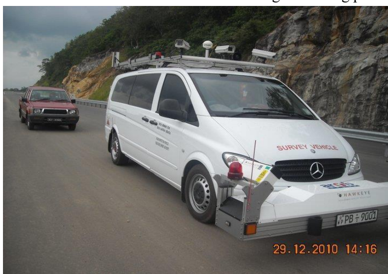
Figure 3. Overview of Hawkeye 2000 Network Survey Vehicle (Source: RDA( 2010))
