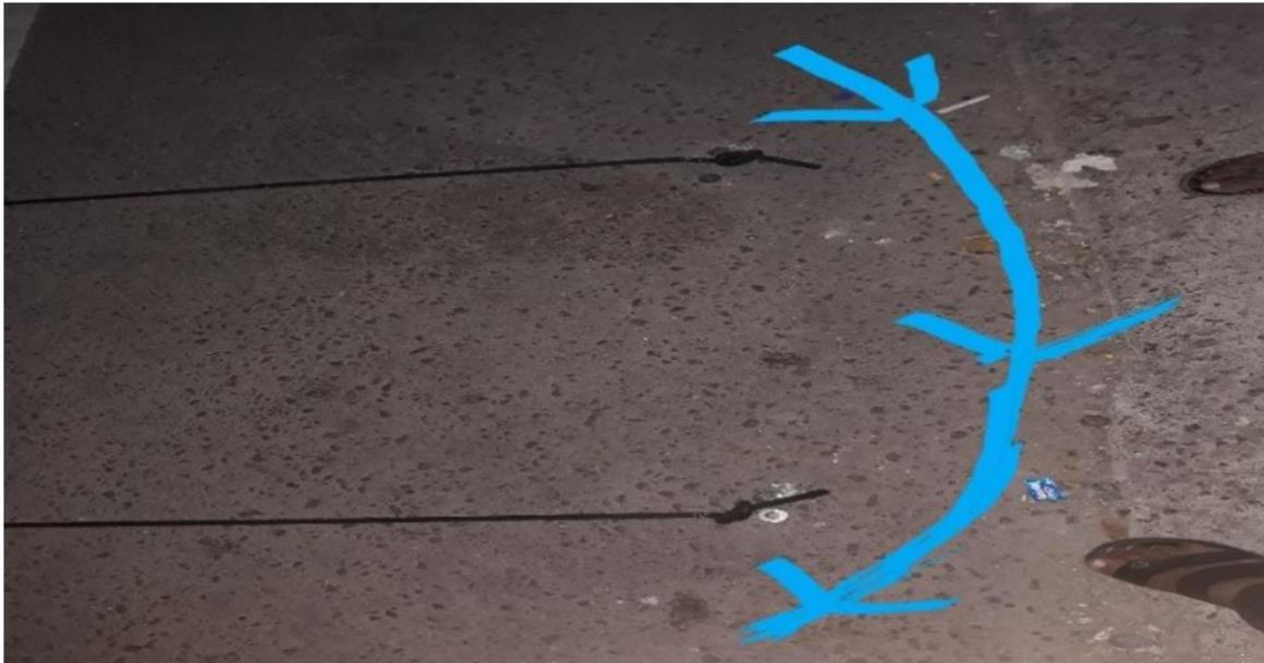
Figure 3. The path follows by some motorcycles avoid recording the counters
