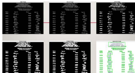
Fig. 2: Apply Pre-processing Techniques for Scanned Attendance Sheets
