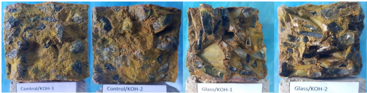
Figure 6. Concrete specimens cured in 1M KOH (Batch 2)
