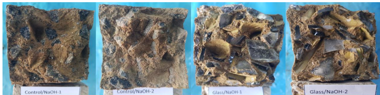
Figure 4. Concrete specimens cured in 1M NaOH (Batch 2)
