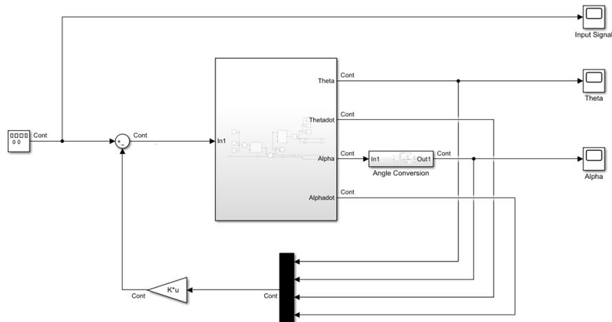
Figure 5. Non-linear Model Controlled using LQR gains
