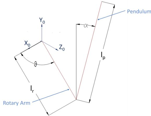
Figure 1. Conventions for Rotary Inverted Pendulum (Inc., 2011)
