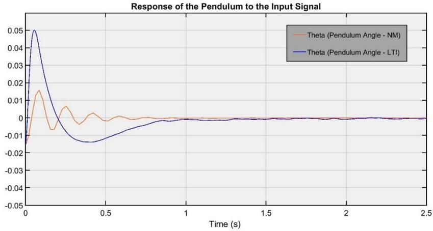
Figure 9. Response of the Pendulum for the Input Signal Case 1 (LTI and Nonlinear Models)
