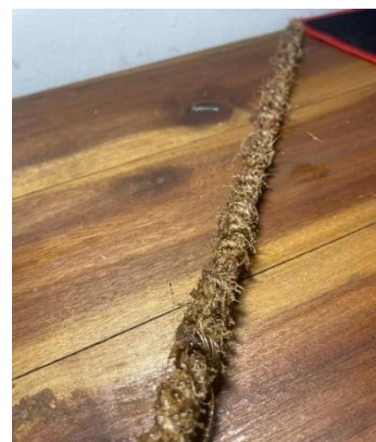
Figure 4- sand coated hardened Coir Bar
