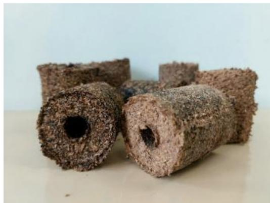
Figure 3. Holey cylindrical briquettes
