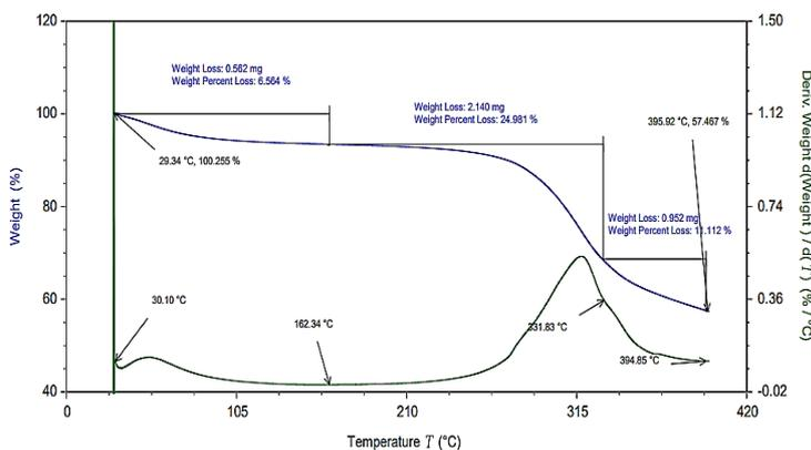
Figure 5. The TGA of rice husks under a nitrogen (N<sub>2</sub>) atmosphere
