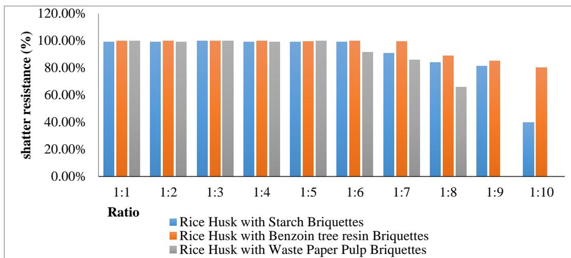
Figure 8. Shatter resistance of the briquettes with different binding agents
