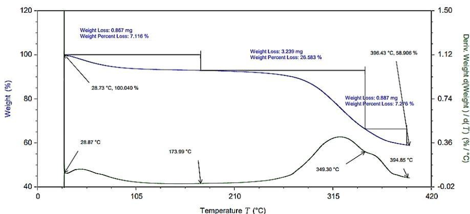
Figure 6. The TGA analysis of rice husks under an oxygen (O<sub>2</sub>) atmosphere
