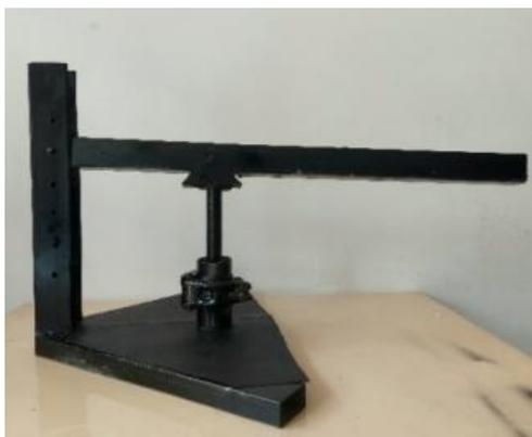
Figure 2. Hand-operated briquette machine
