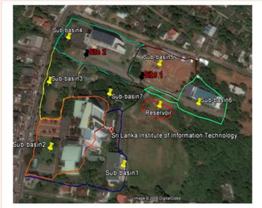
Figure 3A: Basin area divided into smaller basin area sub basins and identified LID installation.
